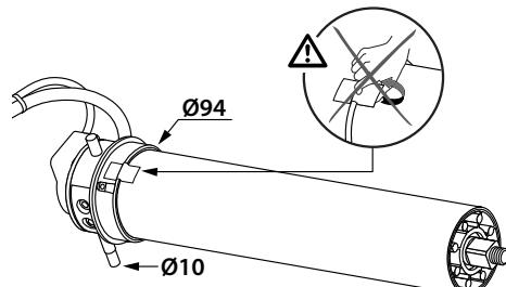
**MONTAGE DES ADAPTATIONS - MOUNTING THE ADAPTORS - ADAPTERMONTAGE****MONTAGE VAN DE ADAPTIJES - MONTAJE DE LAS ADAPTACIONES****MONTAGEM DOS ADAPTADORES - MONTAGGIO DEGLI ADATTATORI - ترکیب المحوّلات****Ø94**
