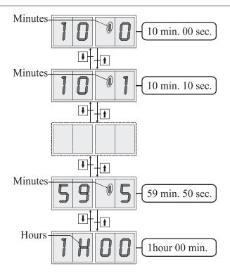
Between 1 min and 10 min press the button or to increase or decrease the timer by 5s.
