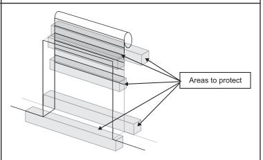
Risk of crushing between the ground and the lower edge of the door during closing.
