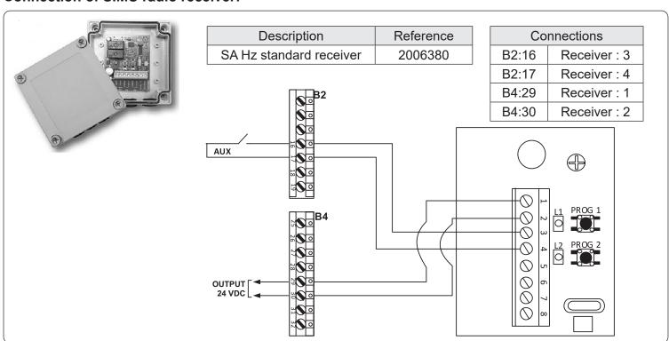
d₂ : Step by step command allows to control the shutter from a SIMU remote control (installation of the SAHz receiver below).
