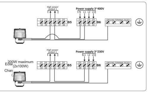
When all wirings are done, replace the protective cover before powering on.
