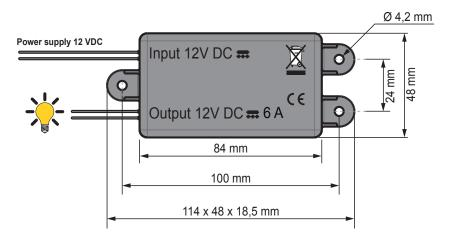
POWER SUPPLY 12VDC (min.: 11V/max.:16V)
